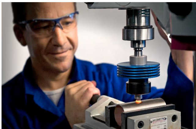
Fig. shows the first step to produce a bushing by thermal drilling.
