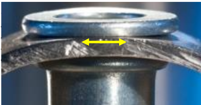
Fig. shows a rivet nut that is crimped to a stainless steel tube with 2,0 mm wall thickness. The yellow arrow shows the small contact area which reduces the holding torque
