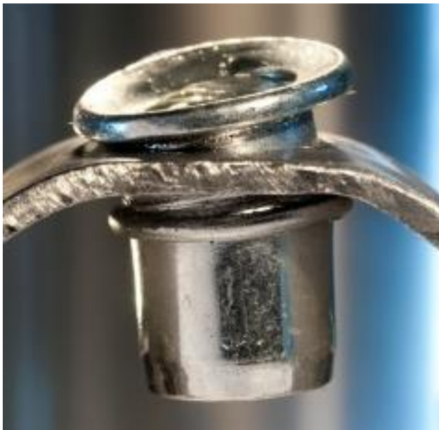
Fig. shows a rivet nut that become loose after load
