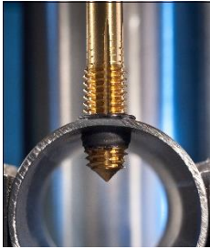
Fig. shows the chipless process of thread forming
